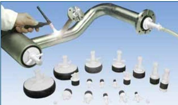
ARGWELD® PIPE PURGING PLUGS ARE USED ON SMALLER DIAMETER (1/2" TO 6") AND SHORTER LENGTH TUBE OR PIPE APPLICATIONS. GREAT FOR SEALING OUTLETS WHEN PURGING VESSELS, AS LOW PRESSURE TEST PLUGS FOR PIPE JOINTS, OR TO STOP CONTAMINANTS FROM ENTERING TUBING. MADE FROM HIGH QUALITY NYLON, THESE PLUGS WON'T RUST OR CORRODE, ARE VIRTUALLY SHATTER PROOF, AND RESIST MANY CHEMICALS.
