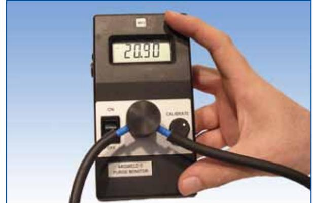
ARGWELD® PURGE MONITORS DETECT THE LEVELS OF OXYGEN IN PURGING GAS TO INDICATE WHEN IT IS AT A SAFE LEVEL TO WELD.
