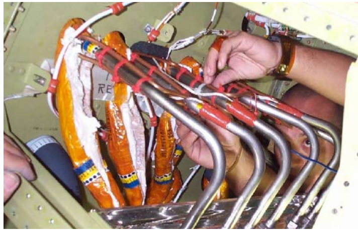
Setting up to freeze multiple lines.
